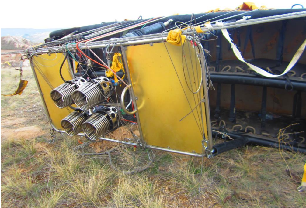
Picture-4: Load Tapes Damage
