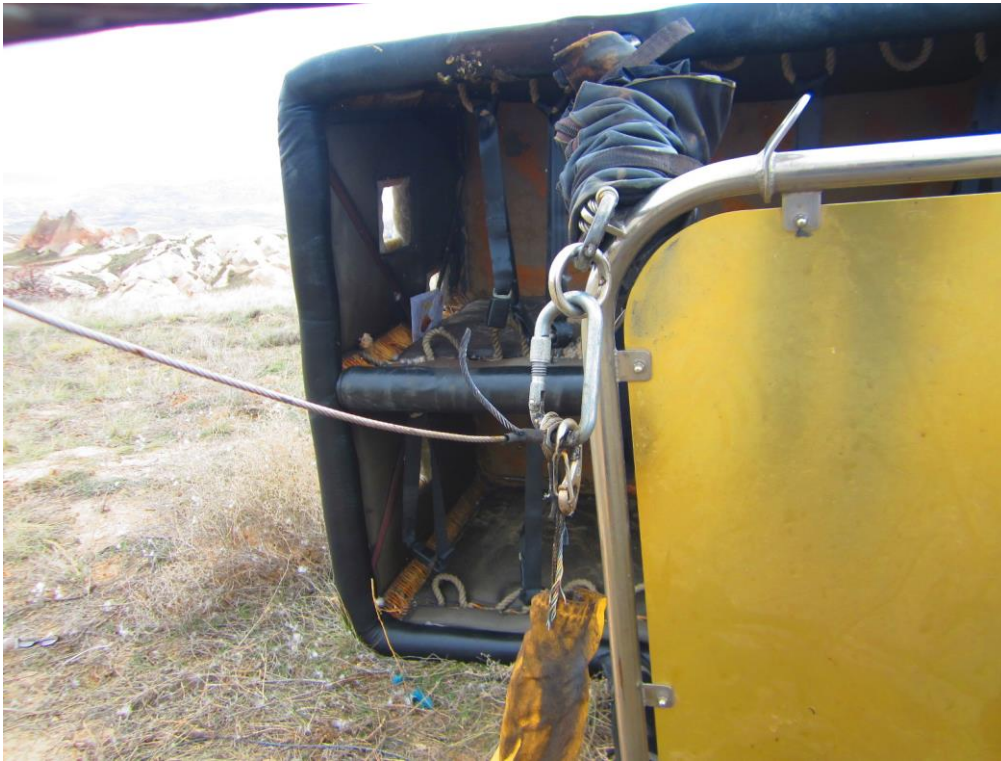
Picture-5: Basket Upper Side Damage
