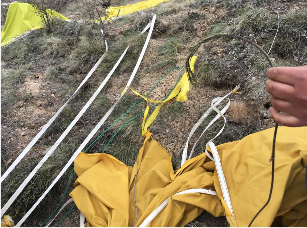
Picture-3: Envelope Load Tapes Damage
